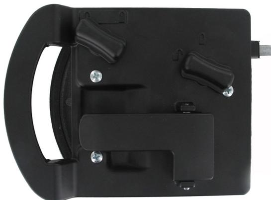
Designed for motor home and fifth wheel trailer entrance doors, this new product is a redesign of our 030-1000/030-1050 Motor Home Entrance Door Hardware. It features easy installation through sandwich mounting, a reliable direct release rotary latch which is compliant to FMVSS 206, a built-in deadbolt for additional security and is power lockable.
